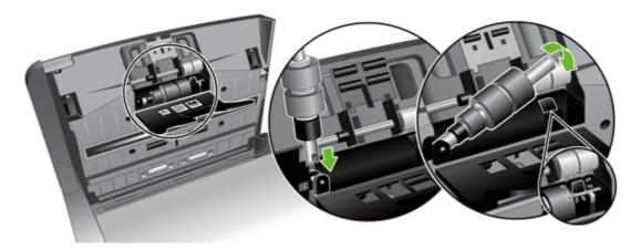
6. Open the door on the inside of the product, open the roller covers, and then remove the rollers.
